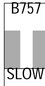
The system goes into "downgrade" mode due to bad weather conditions, pilot will be promoted to slow down. Docking process will continue when the aircraft is detected but pilot should exercise caution
