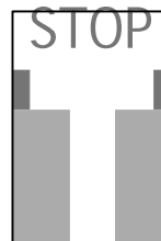
Pilot to stop aircraft when "STOP" is displayed
